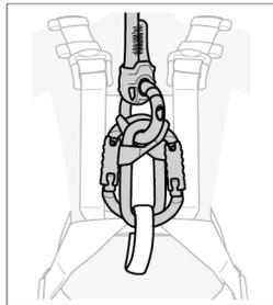
**6b. Tying in with a figure-eight knot**
