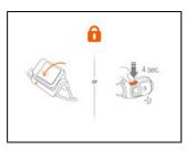
Two LOCK functions to avoid accidentally turning it on.
