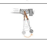
Because the the system allows the carabiner to pivot, the trolley remains in position on the cable when it makes contact with the end brake of the zip line.
