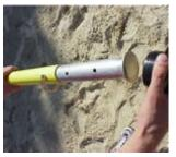
2. Attach the aluminium bottom with the plug to the lower end of the bottom pipe. Now choose the net height by using one of the three borings on the aluminium bottom,
