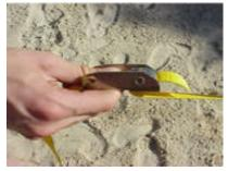
you get four tensioning belts. Put the **small loops** of the tensioning belts underneath the disk of the sand anchors.
