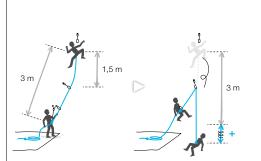
Test conditions Climber: 80 kg Belayer: 80 kg Rope length: 3.6 m Fall length: 3.6 m Rope : VOLTA 9.2 mm (Impact Force: 8.6 kN) Belay device: GRIGRI 2
