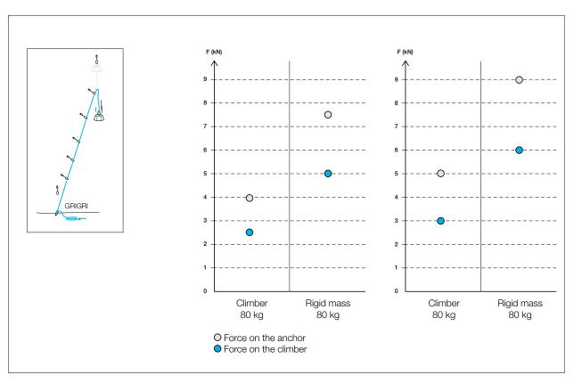
These tests revealed very significant differences between the two protocols: the force on the climber increases by up to 70% with a rigid mass.
